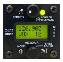
Press the mode switch until the VOX adjust screen is displayed, and set the VOX threshold to the desired level. It may be necessary to readjust this level when the aircraft is operating at full power.
