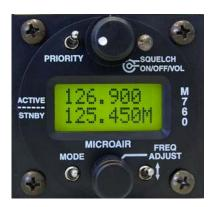
While receiving a signal on the active frequency - the standby channel is **NOT** monitored.
