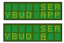
The **blank** option allows the user to enter a three character service description. Scroll top the blank option and press the frequency adjust knob **briefly** to access the editing cursor.
