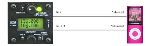
The auxiliary audio input is mono. Most music sources will have a stereo output consistent of left (L) and right (R) audio channels. L and R audios must be combined before connection to pin 6 of the M760Q.
